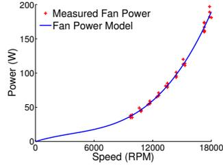
Figure 3. Fan Power Model
