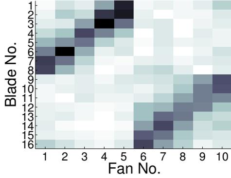
The darker the shade of gray in the above heatmap, the stronger the effect each fan has on the corresponding blade. For example, changing the speed of fan 1 will have a much higher effect on the temperature of blade 8 than blade 1.
