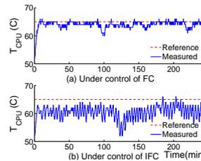
Figure 11. IFC vs. FC: Temperature trajectories of Blade #1
