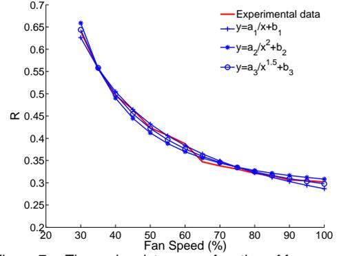
Figure 7. Thermal resistance as function of fan speed
