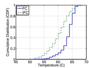
Figure 12. IFC vs. FC: Temperature distributions of all blades
